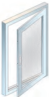
Hinged windows can open inward or outward.
